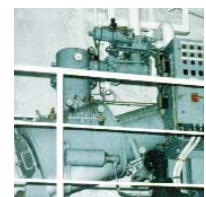
The IGS can be supplied with a topping up Inert Gas Generator with a standard capacity of 500 m 3 /h.
